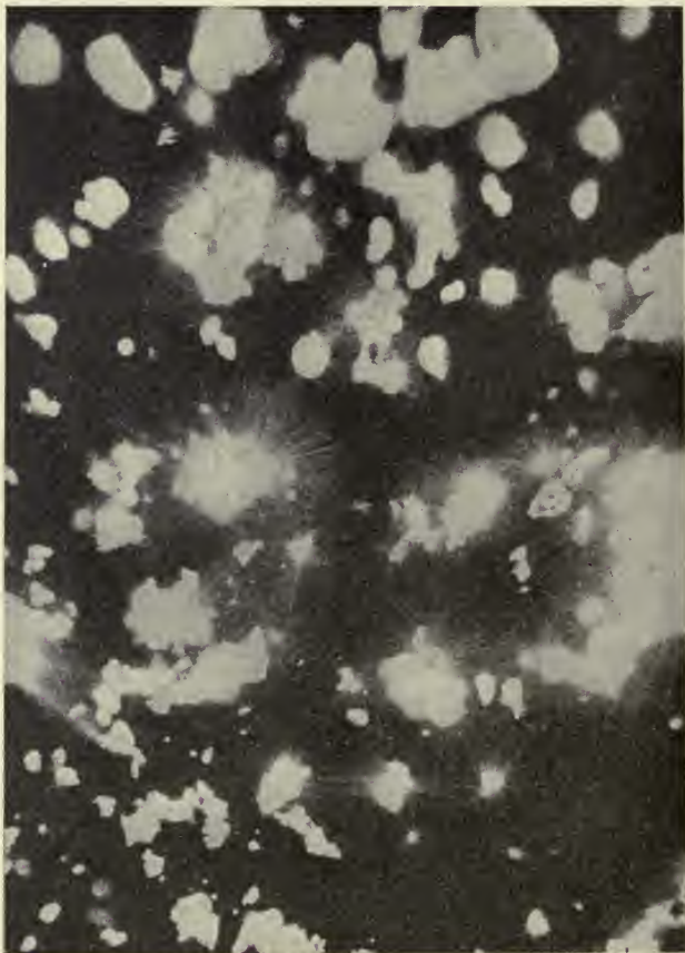
FIG. 45. — Ultramicroscopic photograph of cement in the process of setting, according to H. AMBRONN. Observe the delicate crystalline needles protruding from the gel envelopes.
